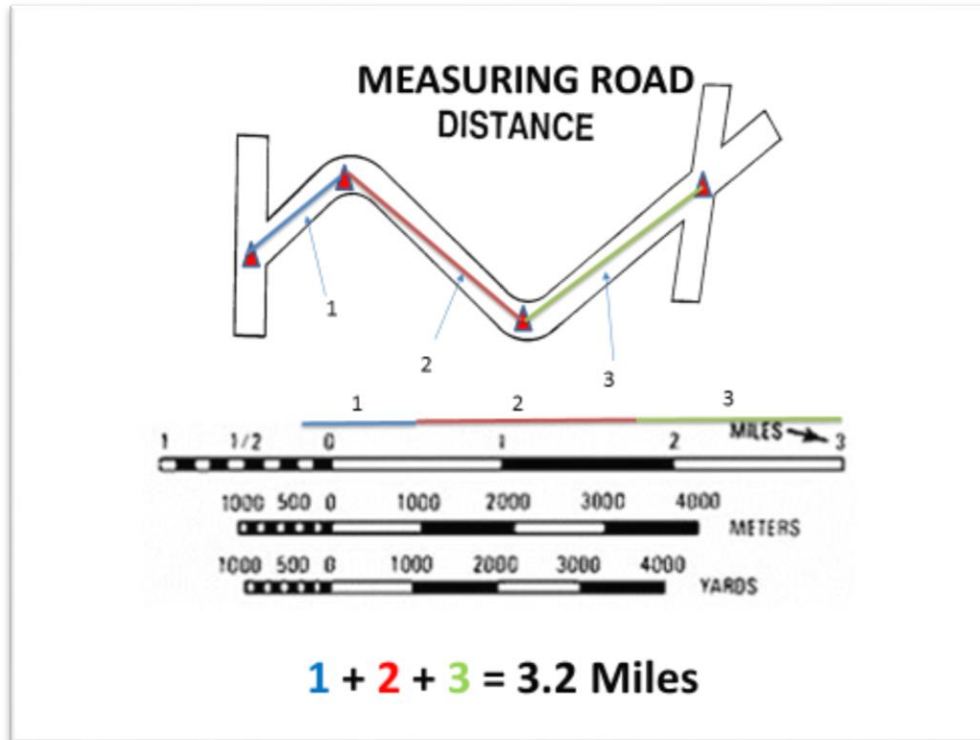
Figure 41 Measuring Distance Along a Crooked Path
